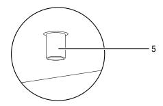
It is impossible to use the device unless the tilt protection switch (5) was pushed entirely into the device. This occurs automatically when placing the device on suitable ground.
