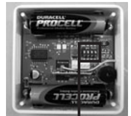
b) Radio sensor circuit board
