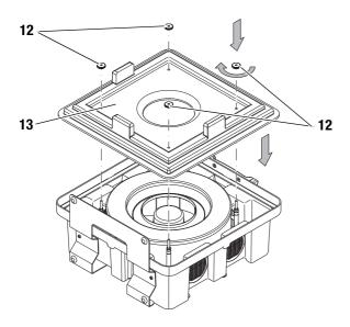
10. Install the new air filter. In doing so, pay attention to the correct alignment (front/rear).
