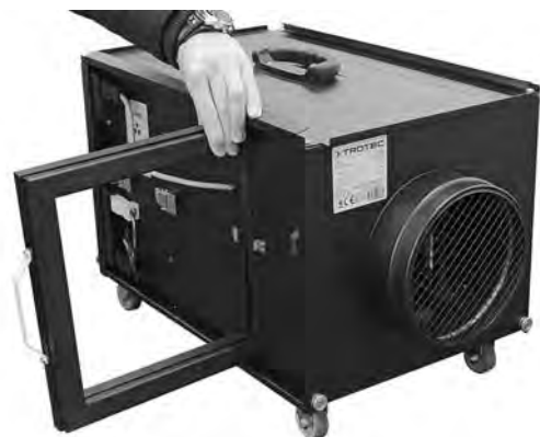
Fig. 4 Removing the tensioning frame
