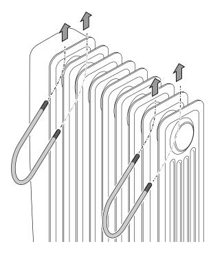
Attach the mounting plates with the castors to the U-bolts. In doing so, observe the position of the cut-outs at one side of the mounting plates. They should be directed towards the device front (control panel).
