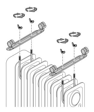
Bolt the mounting plates, wing nuts and U-bolts together.
